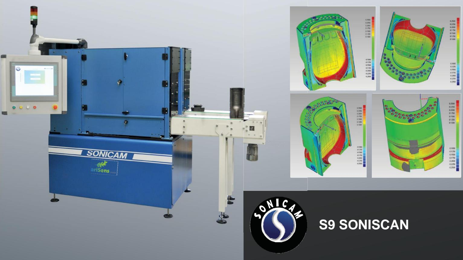
**Sonicam S9** provides automatic 3D scanning measurements of blank, finish moulds and bottles.
